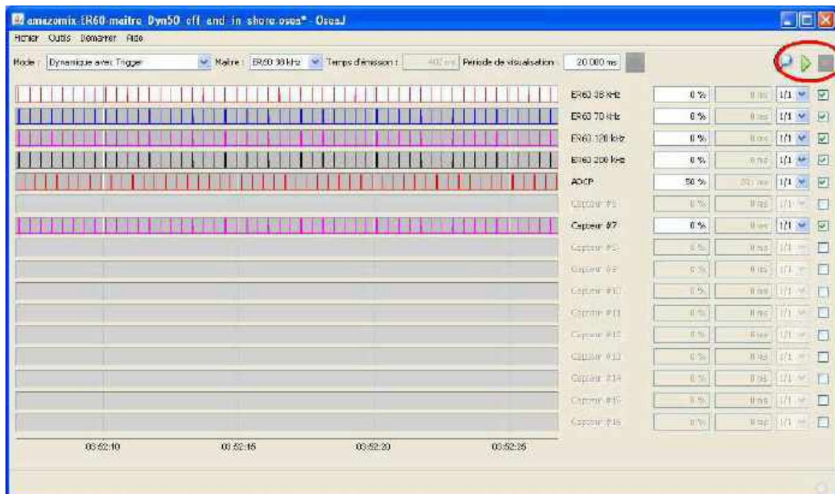
Figure 24. Configuration of OSEA V4.1 software to synchronise the echosounders and the ADCP.
