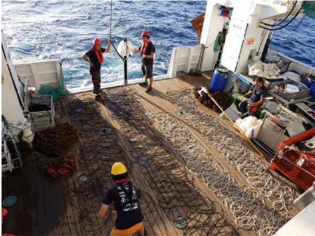
Figure 4. More than 1000 m of rope tether flakes out on deck of Antea before a deep VMP profile.
